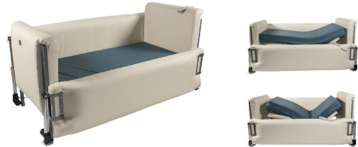
The Novacorr Huntington's Bed (patent pending) is a fully adjustable hospital bed with electrically controlled padded protective side rails. The side rails have a range of 350mm - from 90mm below the height of the mattress (in the raised position) to 460mm above.
